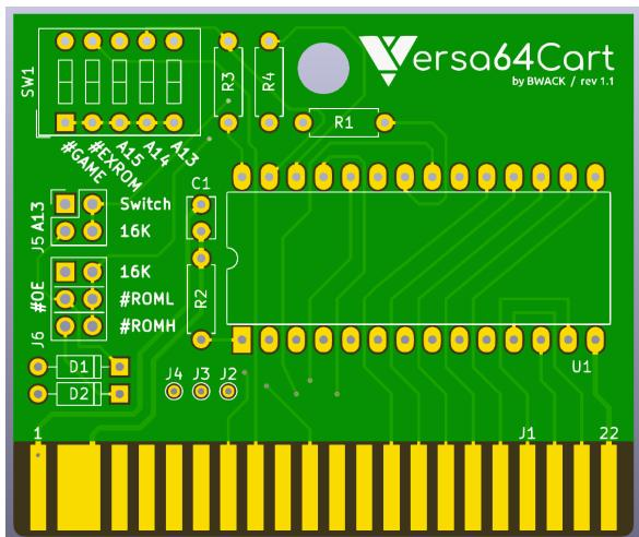
(\*) CAUTION: Only make DIP switch changes when computer is power off. Never change DIP switch settings while cartridge is inserted and computer is powered on.
