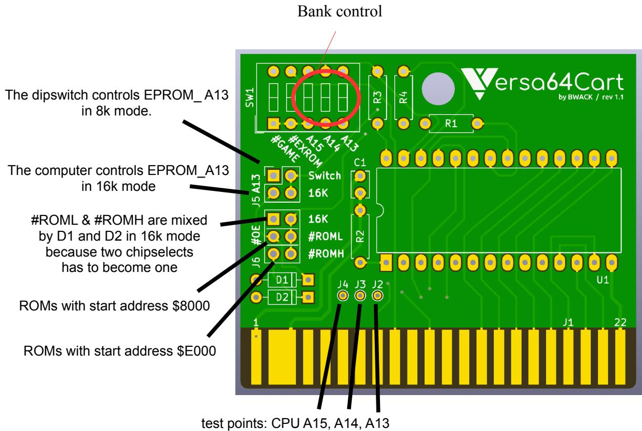
Technical note: The Versa64Cart makes it possible to run 2x8k (16k) ROM games on a single 16k EPROM device. Two chipselects has to become one, and the two 8k images has to be banked with A13.
